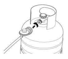
After cooking, be sure to turn off the gas from the gas canister first before turning of the Dome. This will allow any gas left in the burner or pipe to be used up safely. Three minutes after turning the gas off it will be safe to remove the regulator and turn the control dial back to the off position.
