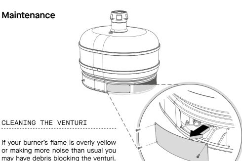
If your burner's flame is overly yellow or making more noise than usual you may have debris blocking the venturi. When the oven is turned off and cool, remove the maintenance hatch and use a vacuum cleaner with a long plastic nose to remove any debris. It's good practice to check the inside of the dock for debris regularly.
